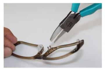
4. Use Frame Barn's FM704 Padded Metal Endpiece Angling Plier to insert the titanium pad arms into the 2 pre-drilled holes.
