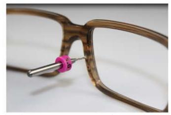
3. Use a marker to locate 2 drill points, then use a 1.0mm drill bit to drill 2 holes on each side. Each 2.00mm deep.
