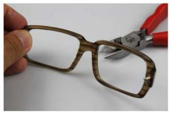
1. Cut original nosepad/plastic pad arm using Frame Barn's FM706 Side Cutter.
